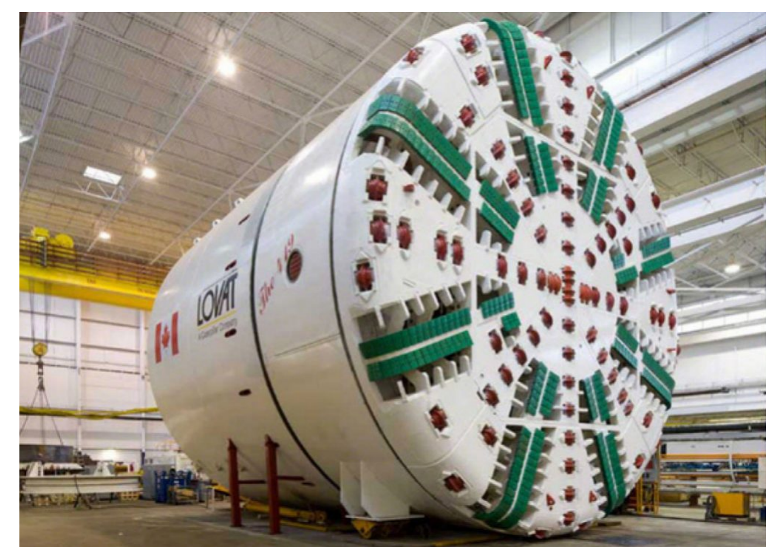
Tunnel Boring Machine (TBM) being used on the Eglinton Crosstown
